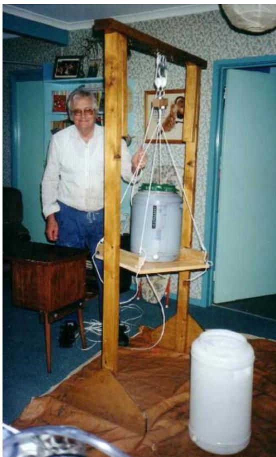
The platform is lowered to the floor, and a 25lt or 30lt container of wine is dragged onto the platform, and then by pulling the rope, the platform is raised high enough to allow me to slide under it a light but strong table that is placed ready, see at the left of the photograph.
